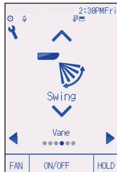
Each pressing of the ▼ or ▲ button cycles through the following vane settings.
