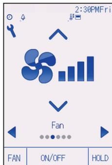
Each pressing of the ▼ or ▲ button cycles through the following fan speeds.
