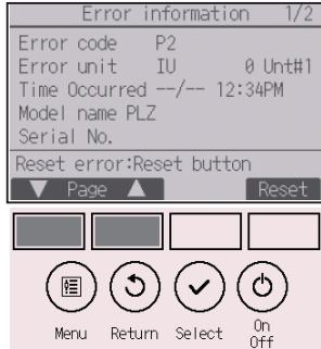
Error code, error unit, refrigerant address, unit model name, date and time on which an error occurred, and serial number will appear.
